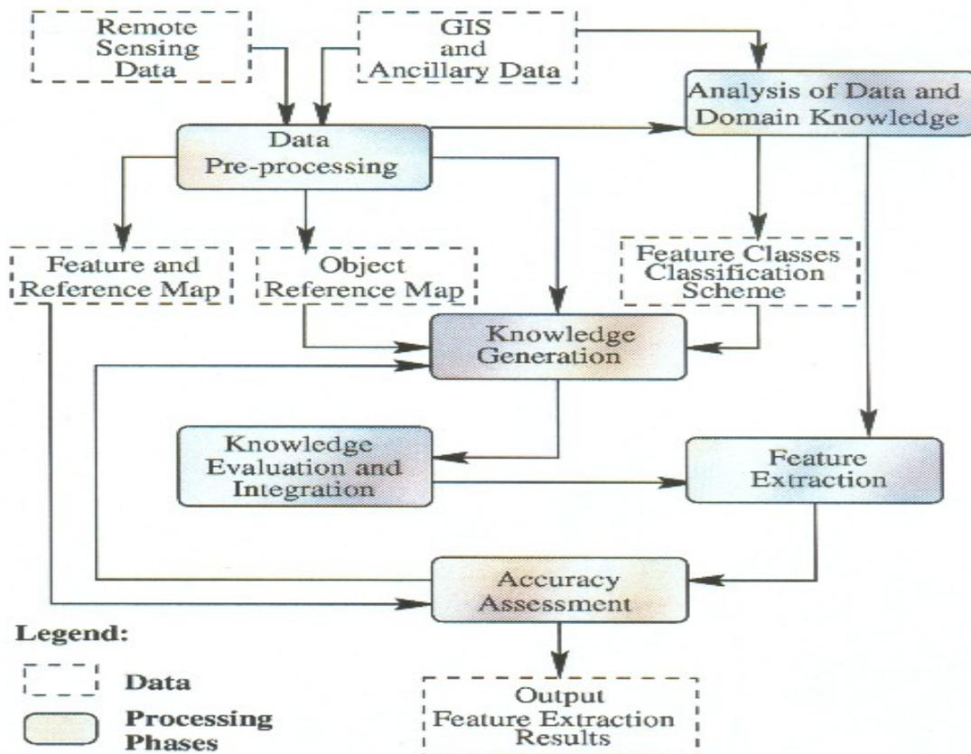
Figure 2 The conceptual diagram of the phases in the methodology of OMIRGS
