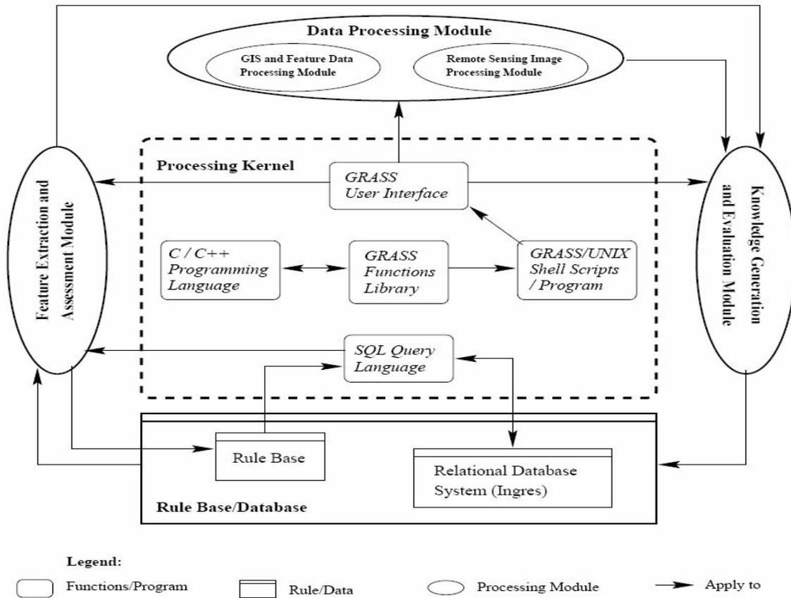
**Figure 3** The system architecture diagram of OMIRGS
